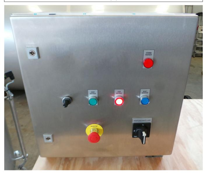
brand new; miscellaneous equipment; SS AISI 304L (V2A); vertical; single-skin: Stainless-steel box 500x500x300; main switch; illuminated start button; indicating light for operation; emergency stop; 24v DC power supply; frequency controller up to 5kW; illuminated stop button; indicating light for malfunction; 3m cable with plug
